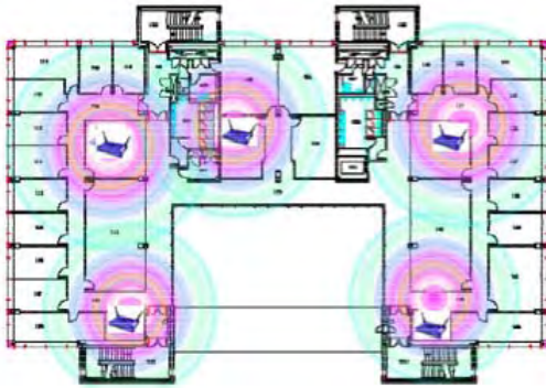
Fig. 1. Schematic diagram showing wireless access point location and expected coverage – second floor of the trial building
